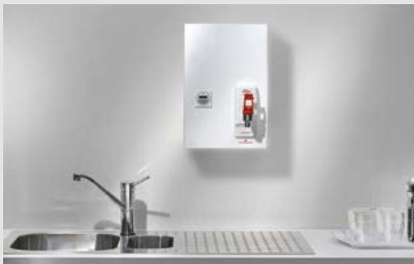
Featuring thermostatic temperature control, a two-way safety tap, twin-chamber boiling technology with stainless steel boiling chamber, plus 24/7 on/off power clock, turning power on/off up to 5 times per day, to meet the requirements of J6.6 of the Building Code of Australia. Zip GlobalPlus 0.2 micron filtration is standard. Three year pro-rata warranty on tank. Two year conditional warranty on heater; first year parts and labour, second year parts only.
