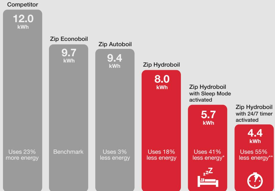
Table shows estimated weekly consumption without provision for water draw-off. Each 176mL cup drawn off = approximately an added 17 watt-hours of power. Estimated power usage is based on continuous operation except where noted.
